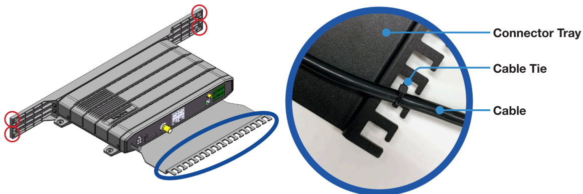
Figure 27: Mount BDU Assembly into 19" Rack
